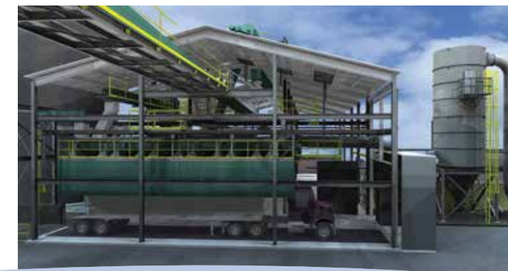
► Truck Loadout with an Aspiration Hood
